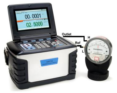
Figure 4 ADT761 calibrator with DUT
